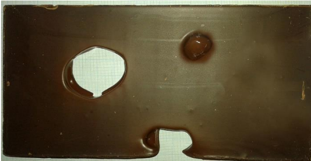
Figure 7. "Imprint" of the anti-nodes of the standing wave on a chocolate bar at a height of z_0 = 2.5 cm
